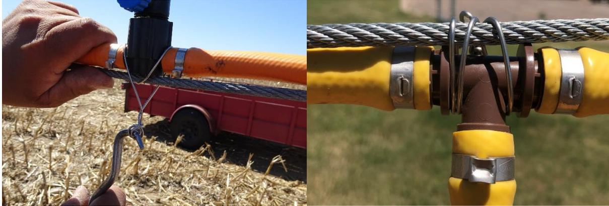
Above you can see how the adaptor tee and tee are secured to the cable
