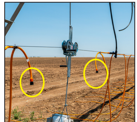
Terminate manifold assembly with #72. Power Lock Plug
