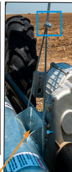
Place Center of winch at 5 or 5 1/2 feet.
