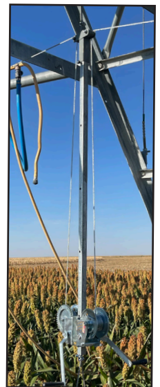
Highline Dual Winch Assy in the field
