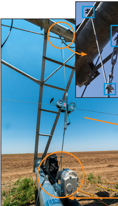
Place Center of winch at 5 or 5 1/2 feet.
